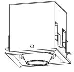
Suitable for Ceiling thickness 5-20mm.
